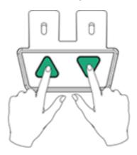
3. Press the **Down** button and lower the stand to the lowest position.
