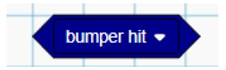
Unlike some of the other sensors, the Bumper Hit block does not need to be seated inside a green **operator**. This is because it is a **boolean** sensor and only has two states (hit or not hit) whereas other sensors have a larger range of potential readings.
